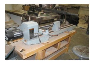
Lathes should be equipped with hoods enclosing the cutter blades completely except at the contact points while the stock is being cut. A hinged shield permits adjustments when needed.
